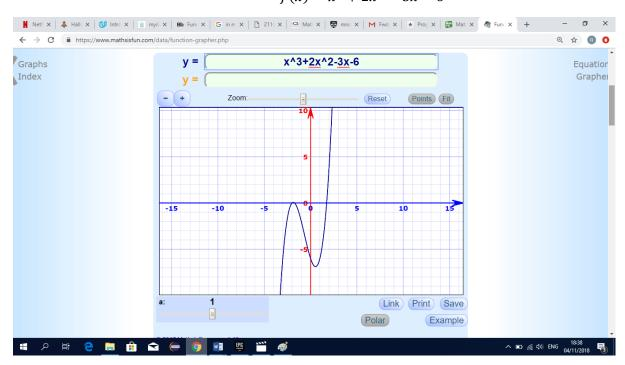
The above function has an index of 3, subtract 1 from this which gives 2. This is a line with 2 turns, hence it must be a sideways "S" shape as shown (eg. A Cubic function).
