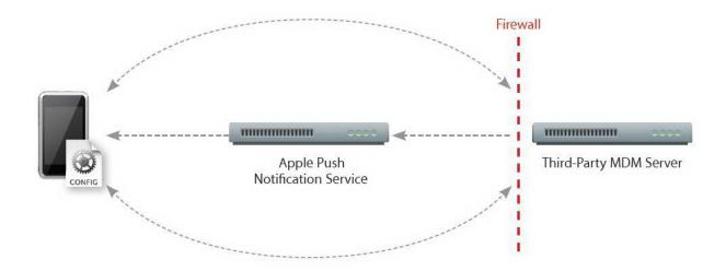
This is how the basic layout of the communication flow looks between a device and the MDM server:
