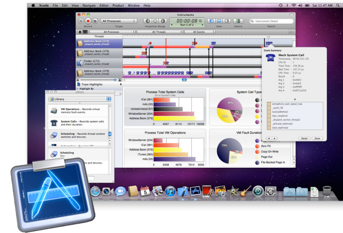
Instruments collects and displays data in real time, such as disk, memory, or CPU usage, making it easy to pinpoint problem areas.
